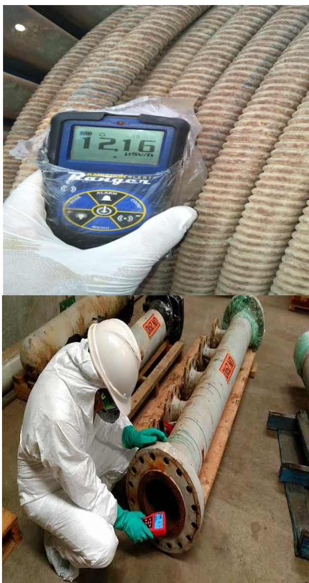
Fig.(13): Typical decontamination activities for vessels and tools and radiation survey before and after decontamination
